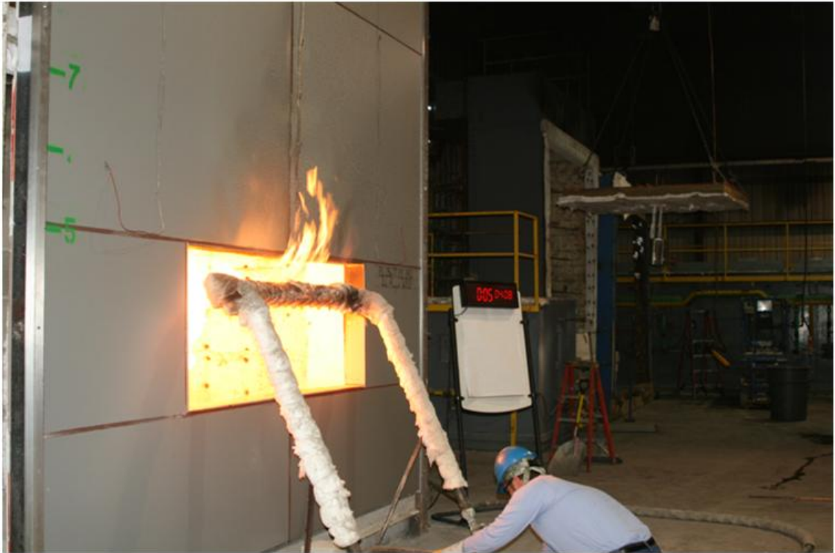
Figure B-3. Application of Window Burner.
